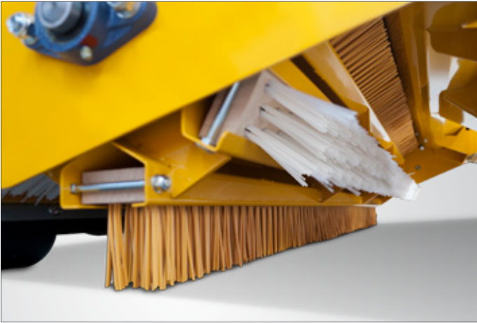
Brushes arranged in a revolving way for different brush hardness.
