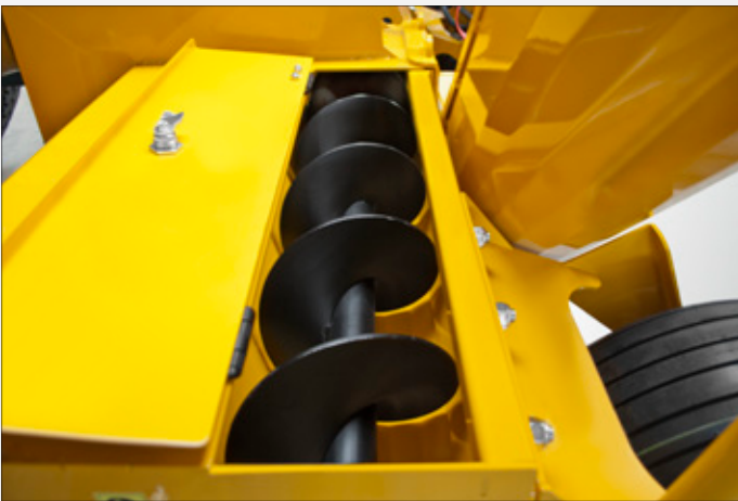
Large sized transport feeding auger for a high flow rate
