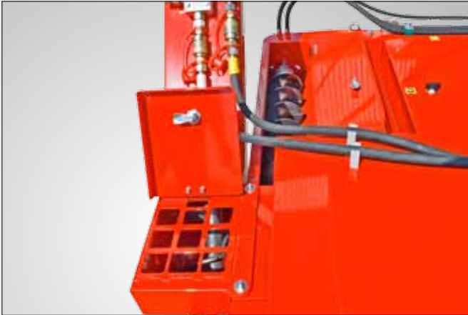
Auger for the transport of the infilling material, speed adjustable.
