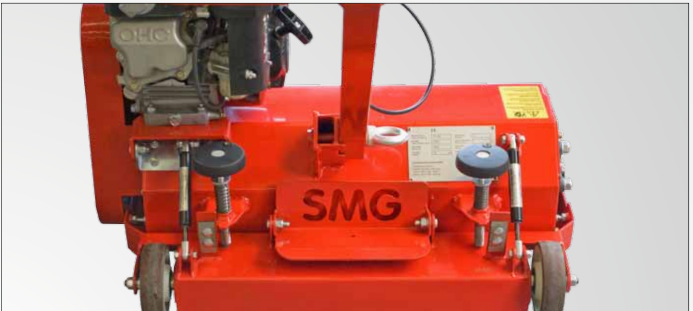
Working depth adjustable via spindles
