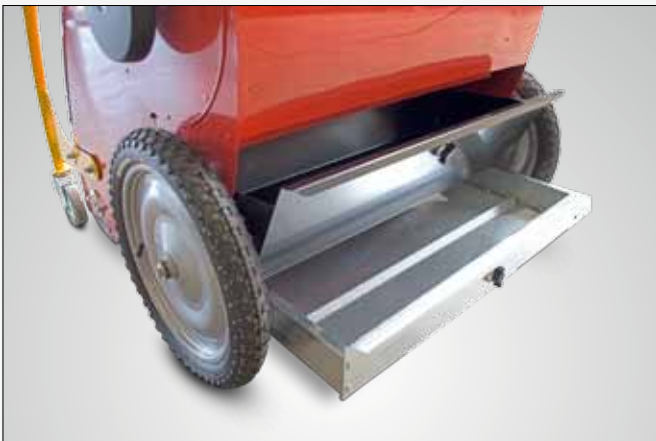
The cleaned granulate is returned to the carpet by the vibrating screen
