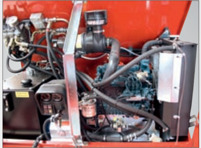
Water cooled 3-cylinder Kubota diesel engine
