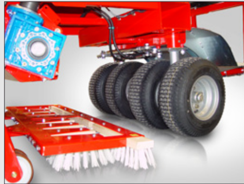
6 large wheels for minimum ground pressure and easy maneuvering
