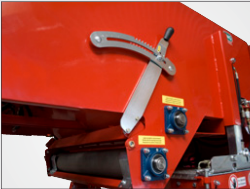
Material output exact adjustable through a slide valve
